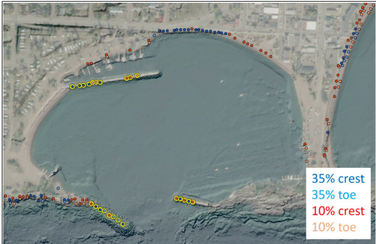
Figure 7. Bluff extraction results shown as blue and red points for two slope threshold parameters of 35% and 10%, respectively. Yellow highlighted features were manually removed during QC as these points were located along coastal structures.
