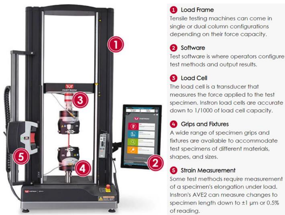
Figure 2. Overview of Universal Tensile Tester [34].
