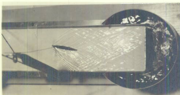
(C) ANGLE OF ATTACK = 10° MACH. NUMBER = 1.94
