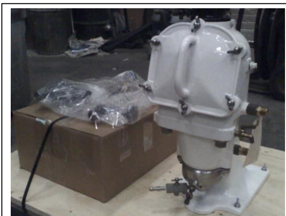
Figure 2: The Sharpley T1P Tubular Bowl Centrifuge.
