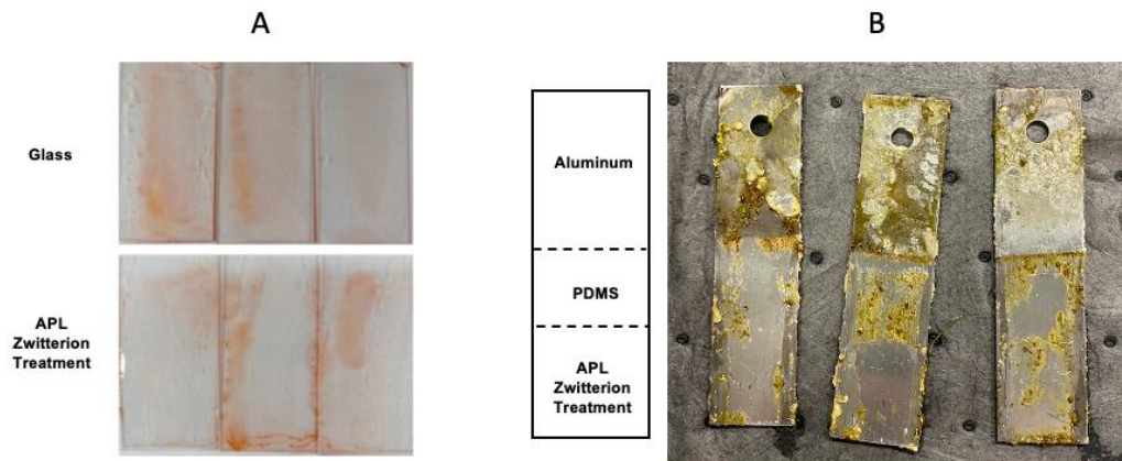
Figure 18. (A) Samples after being exposed to plating of Sulfitobacter in a drip reactor for 72 hours. Samples are stained with Congo Red for visibility. (B) Samples after being exposed to flowing water from a tank with a mixed marine community for 5 days.
