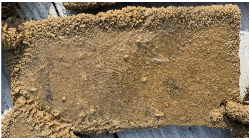
Figure 19. Aluminum panel coated in epoxy after 2-week exposure in the marine environment of SERC. The left side of this panel has been treated with a PZI UV treatment. While not well captured in the photo, fouling was different on the left hand side, compared to the right, indicating that the coating had some influence on biofouling.
