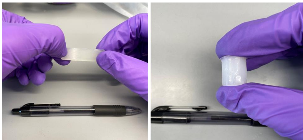
Figure 6: UV-cured (left) and thermally cured (right) final elastomer formulation.
