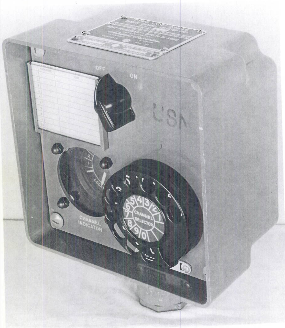
FRONT OBLIQUE VIEW, TYPE CQC-23445 REMOTE CHANNEL SELECTOR UNIT FOR TDZ, RDZ, RDR OR MAR RADIO EQUIPMENT
