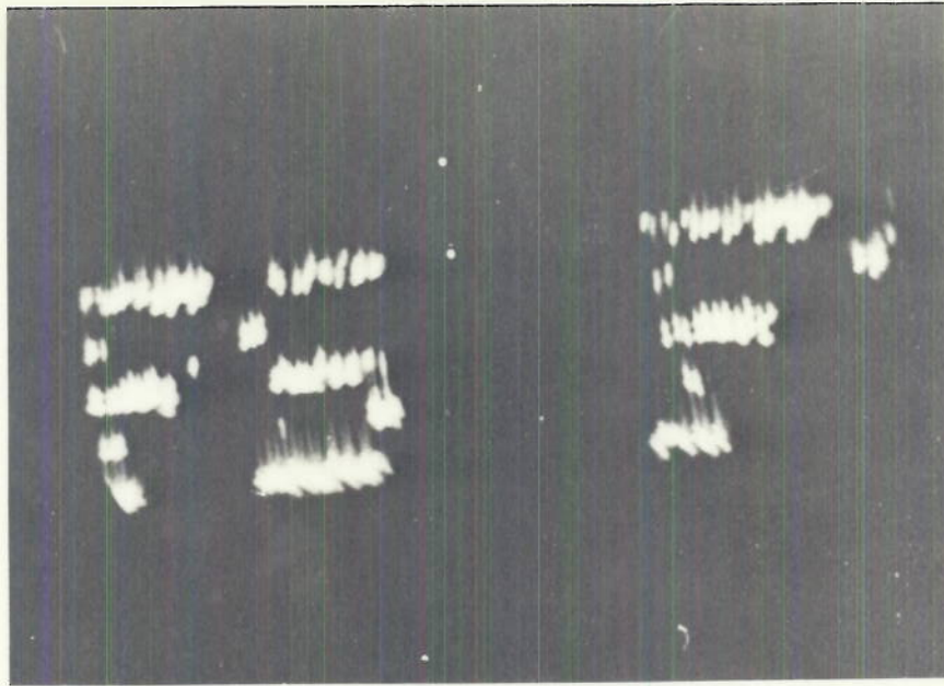
"NARROW" LETTERS "FS" VIEWED ON VF TYPE B INDICATOR RANGE TO TARGET 45 MILES ANTENNA RPM 7, CODER CAM RPM 150
