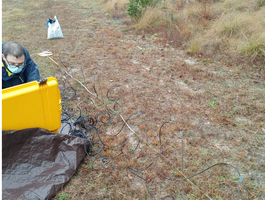
Figure 10: Typical layout of CR field measurements showing electrodes for current injection and voltage recording spaced 0.2 m apart
