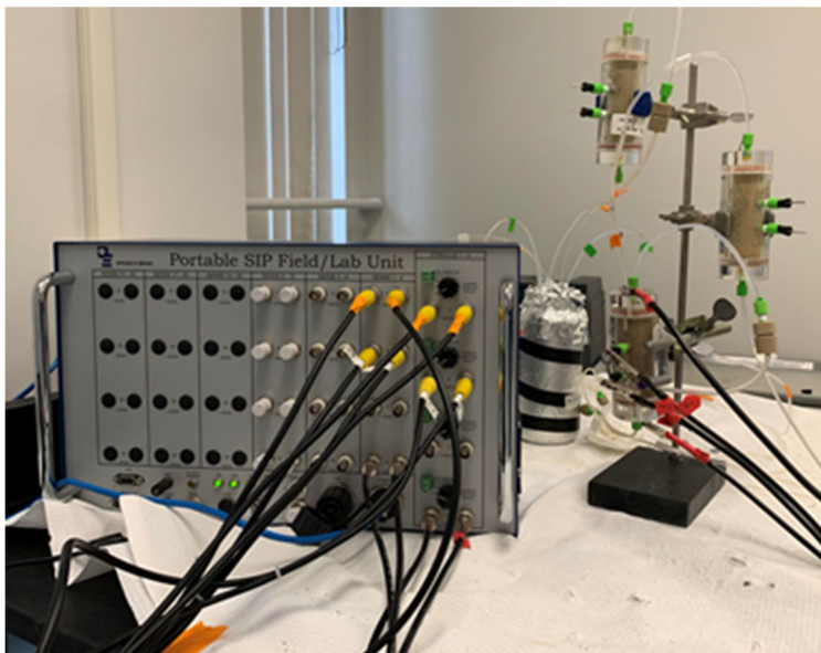
Figure 8: Portable Spectral Induced Polarization (PSIP) for data collection in the foreground, with the triplicate preparations of Sample I1 (a site of known PFAS contamination) shown in the background. Note that the samples were kept in an environmental chamber for the duration of the experiment (the setup shown here is for the photograph only).
