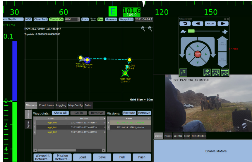
Figure 5. Screen Shot of Greensea Systems EOD Workspace Graphical User Interface.
