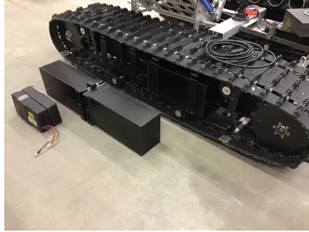
Figure 26. 42 amp-hr Battery Packs Lithium-Ion (Foreground) vs Lithium Iron Phosphate.
