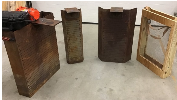
Figure 9. Caisson Designs Tested Include Full Rigid Box, \frac{1}{4} and \frac{1}{2} Scale, Screen and Frame.
