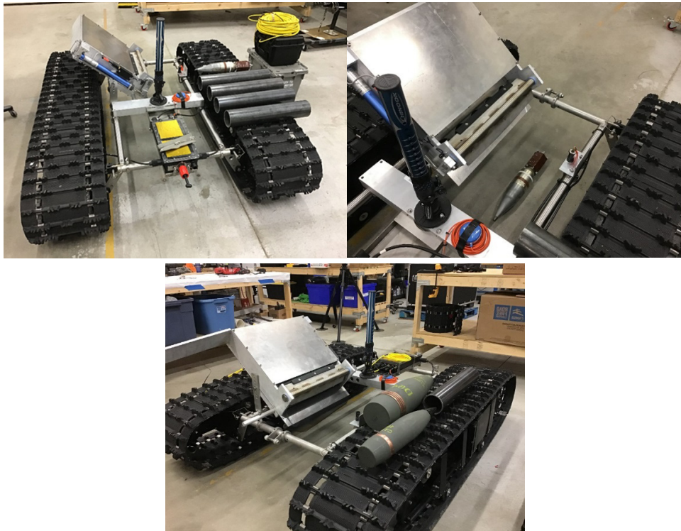
Figure 21. Roll-in-place Dispenser Mounted on Sea Beast.
