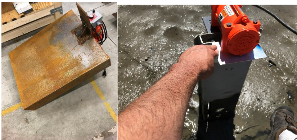
Figure 10. Vibrator Mounted onto the Caisson Boxes.
