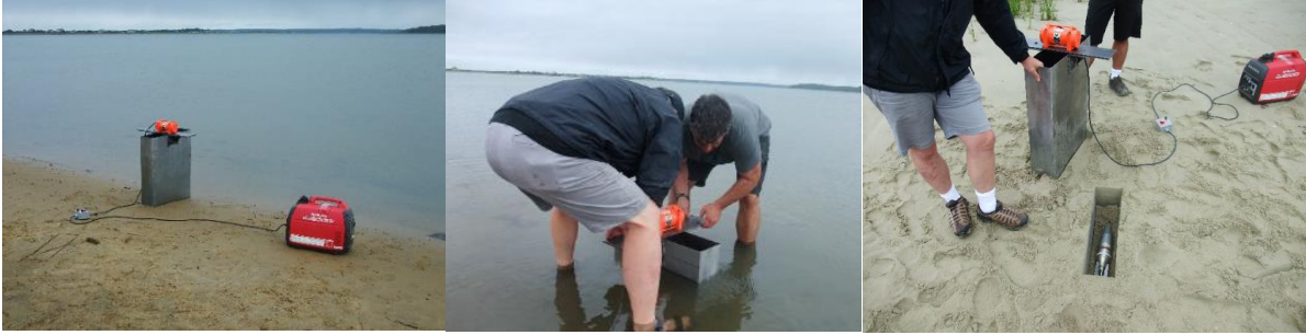
Figure 15. Caisson Testing in Well Graded Sands, AT4 (84-mm) Round Inserted for Scale.
