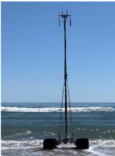
Figure 4. 5-m Mast Mounted on Sea Beast with RTK Receiver.
