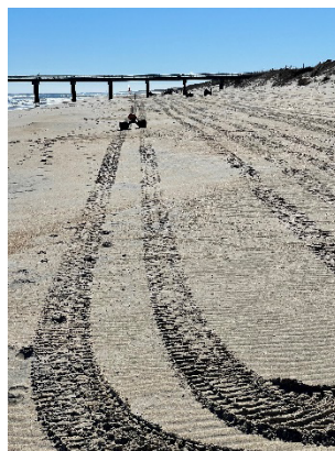
Figure 6. Sea Ox Operating in GPS Denied Conditions, on the Same Track after 1.6km and 12 Turns Transit.
