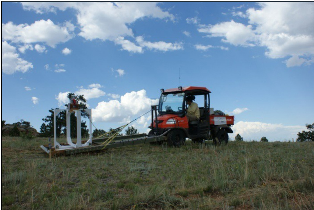
Figure 23. Photograph of the MetalMapper System that Was Used to Collect the AGC Data.
