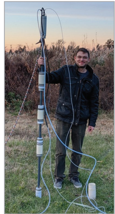
Figure 3. The MI-PET tool ready for a downhole installation. (Source: Courtesy of Rutgers University)
