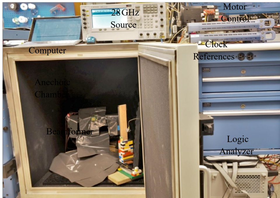
Fig. 4. Over-the-Air Measurement TEST Setup
