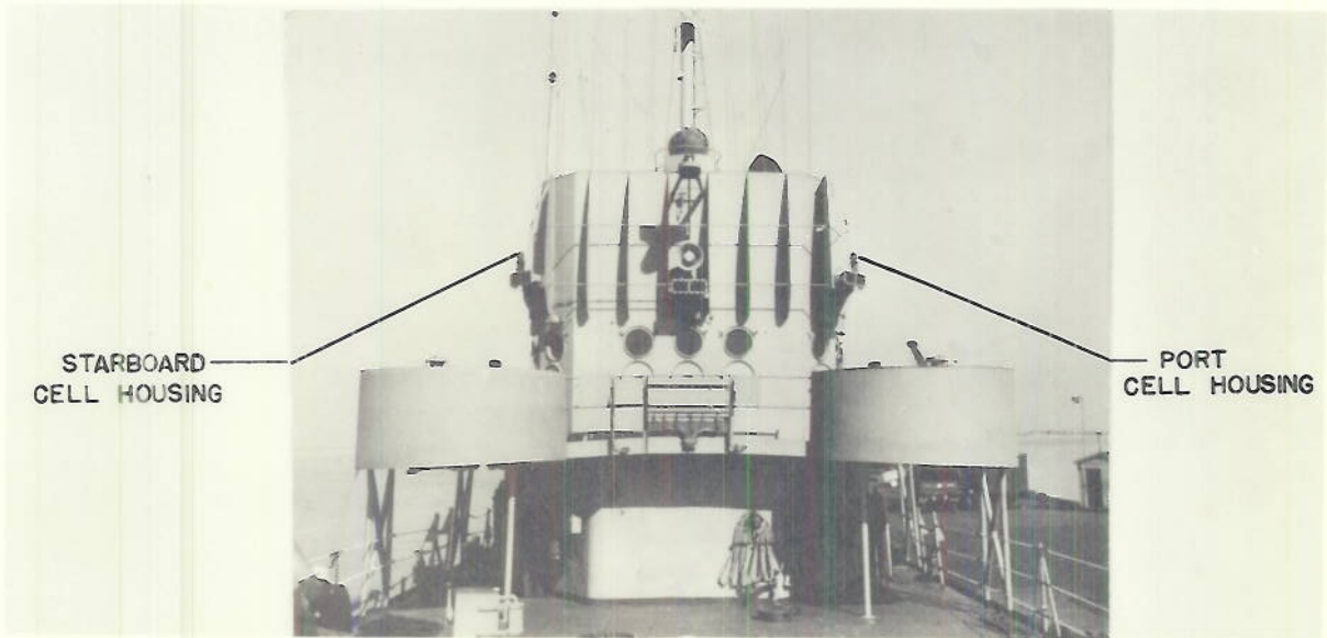
CELL HOUSING INSTALLATION
