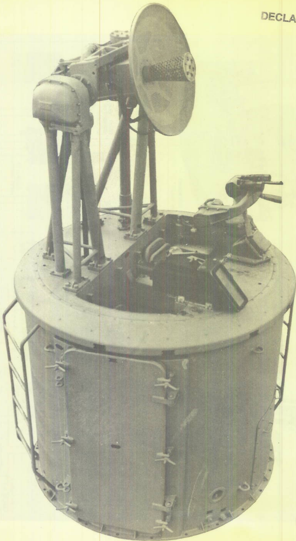
PLATE 2 Mk 61 Director with Eastman 30" Antenna (Front View).
