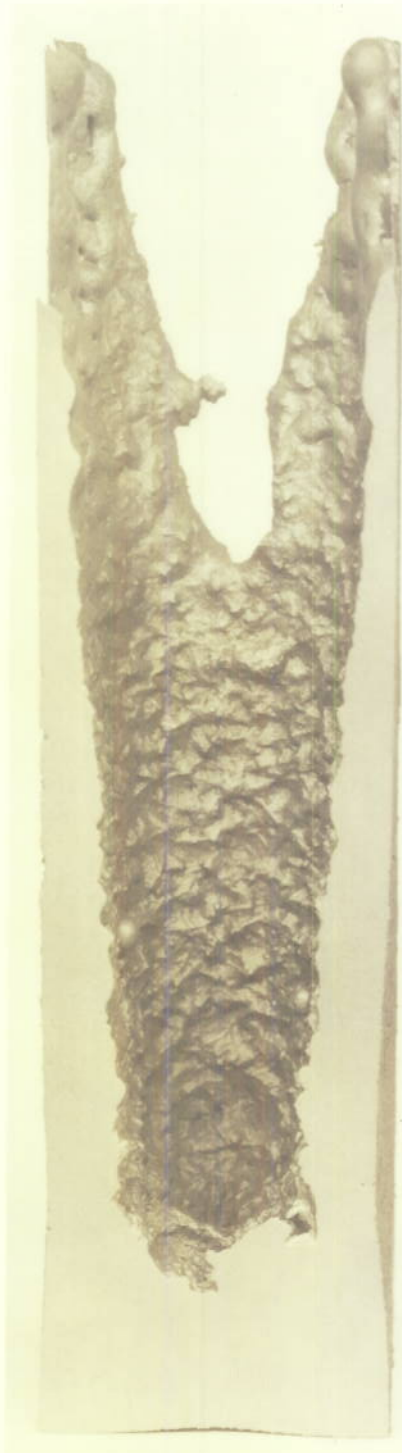
TAPER OF WALL THICKNESS SHOWN IN A CASTING TOP BLED TWO MINUTES AFTER POURING
