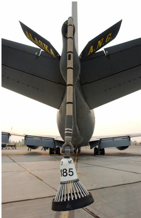
Figure 6.8 BDA Installed on KC-135 Boom
