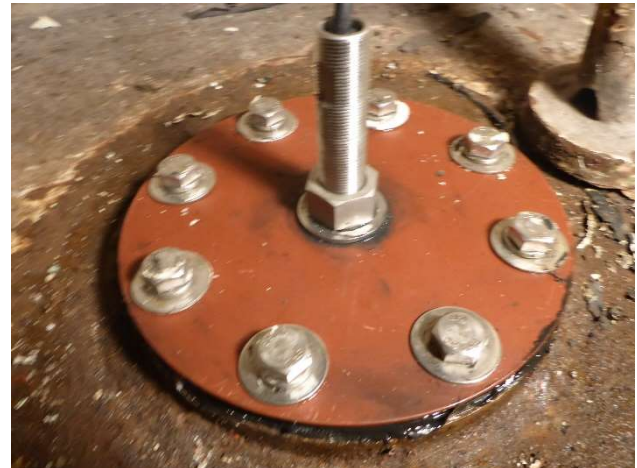
Figure 2. Transducer well on 140' Bay class Icebreaking Tugboat.
