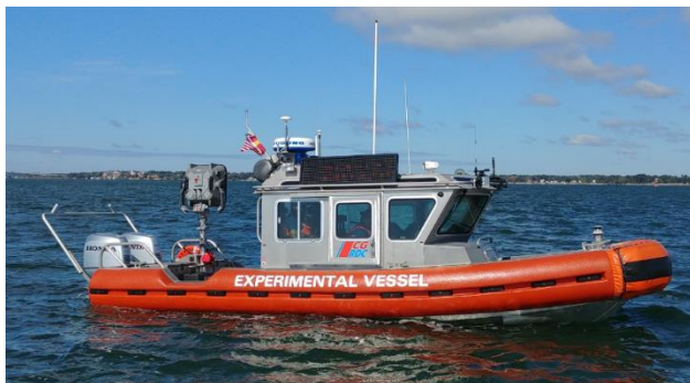
Figure 1. 25417 converted to USV with message sign and LRAD.
