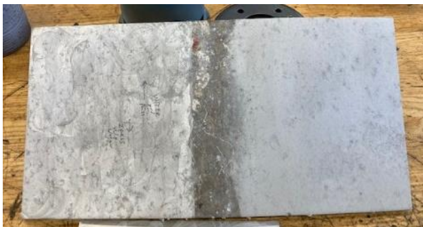
Figure 4. Aluminum plate, center surface corrosion – Left: Laser, Right: Sand blast. (Source: USCG)
