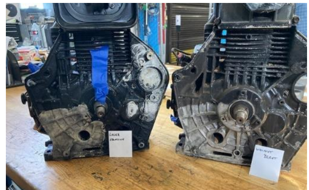
Figure 3. Engine blocks – Left: Laser ablation, Right: Walnut media blast. (Source: USCG)
