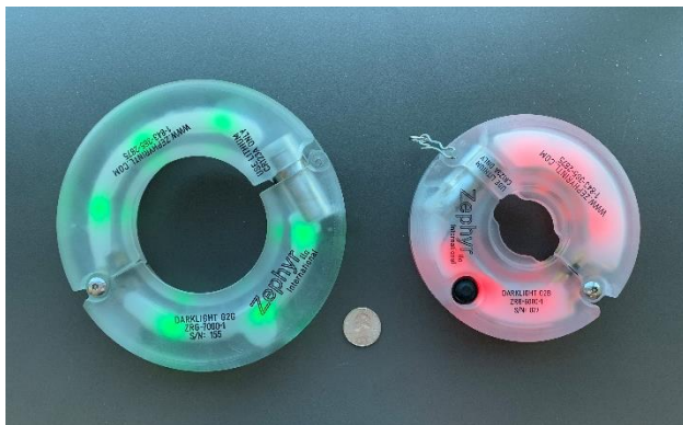
Figure 1. Goodrich (MH-60) Style Light on the Left, Breeze (MH-65) Style Light on the Right. Photo Credit: USCG
