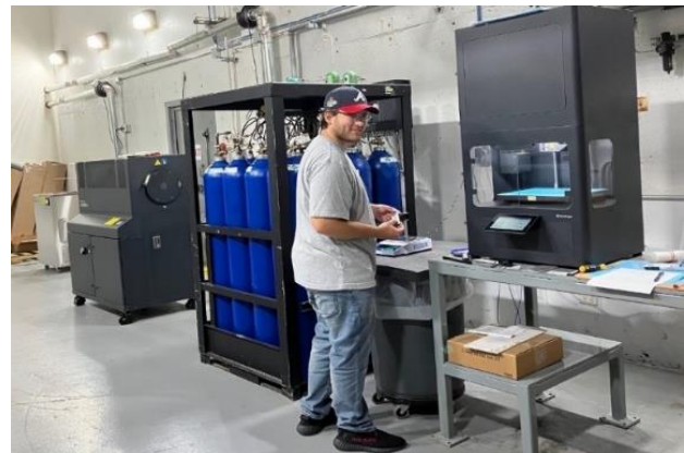
Figure 3. 3D Metal Printer includes three core equipment components. From left to right: Dryer, Sinter Machine, 3D Printer. (Source: USCG)
