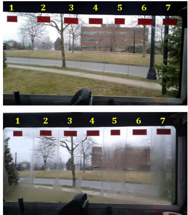
Figure 3. Antifogging product testing on the 29' before (top) and after (bottom) the humidifier was turned on. From left to right the products are: (1) LifeArt, (2) Parker's Perfect, (3) Quick Sheen, (4) Optix 55, (5) Zooke, (6) Z-clear, and (7) a control where no product was used. (Source: USCG)
