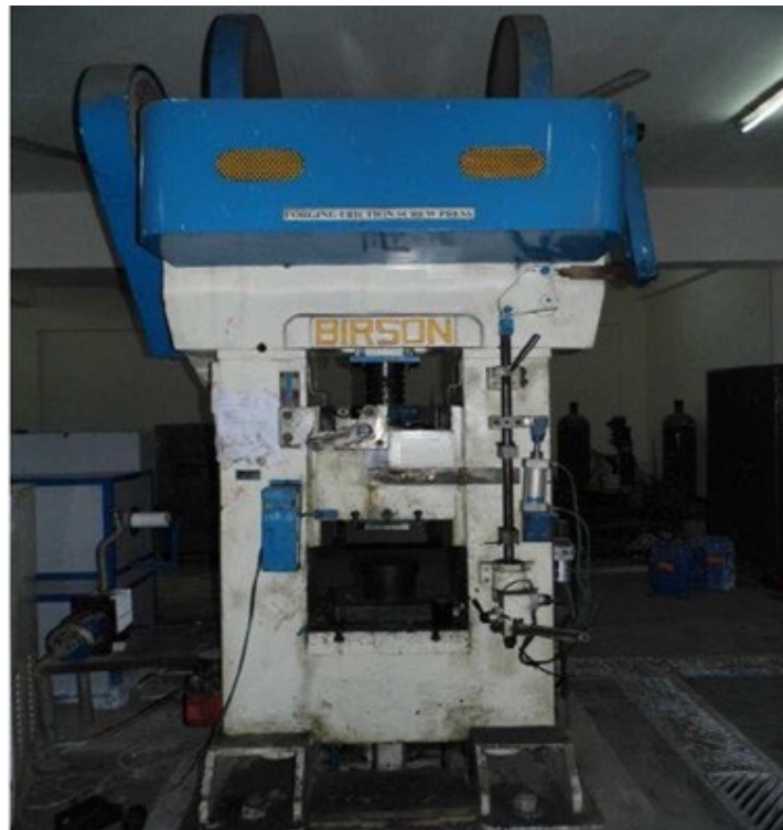
Figure 1. Friction screw forging machine used for Multi-axial forging
