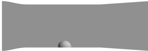
Figure 8: Sideview of the Notre Dame subsonic wind tunnel with turret model
