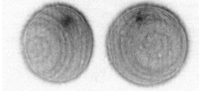
Figure 29. Unthresholded inverted-color upstream and downstream spot patterns for focused Malley probe at a C/L ratio of 20%
