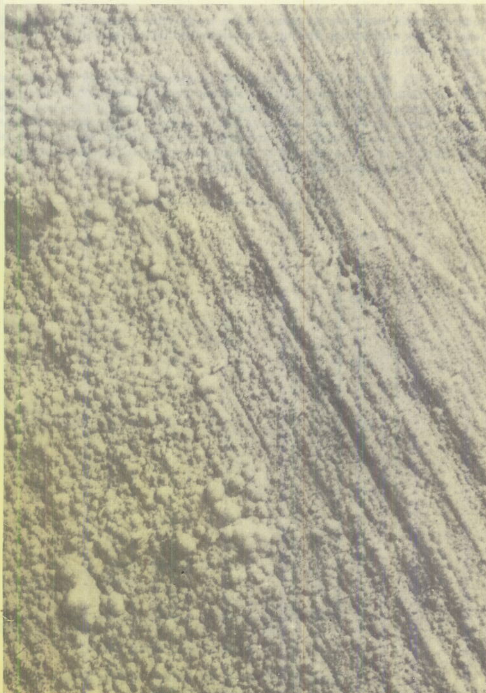
Figure 39 Electron Micrograph of Aluminum Foil Treated with Mixed Chromic-Sulfuric Acids
