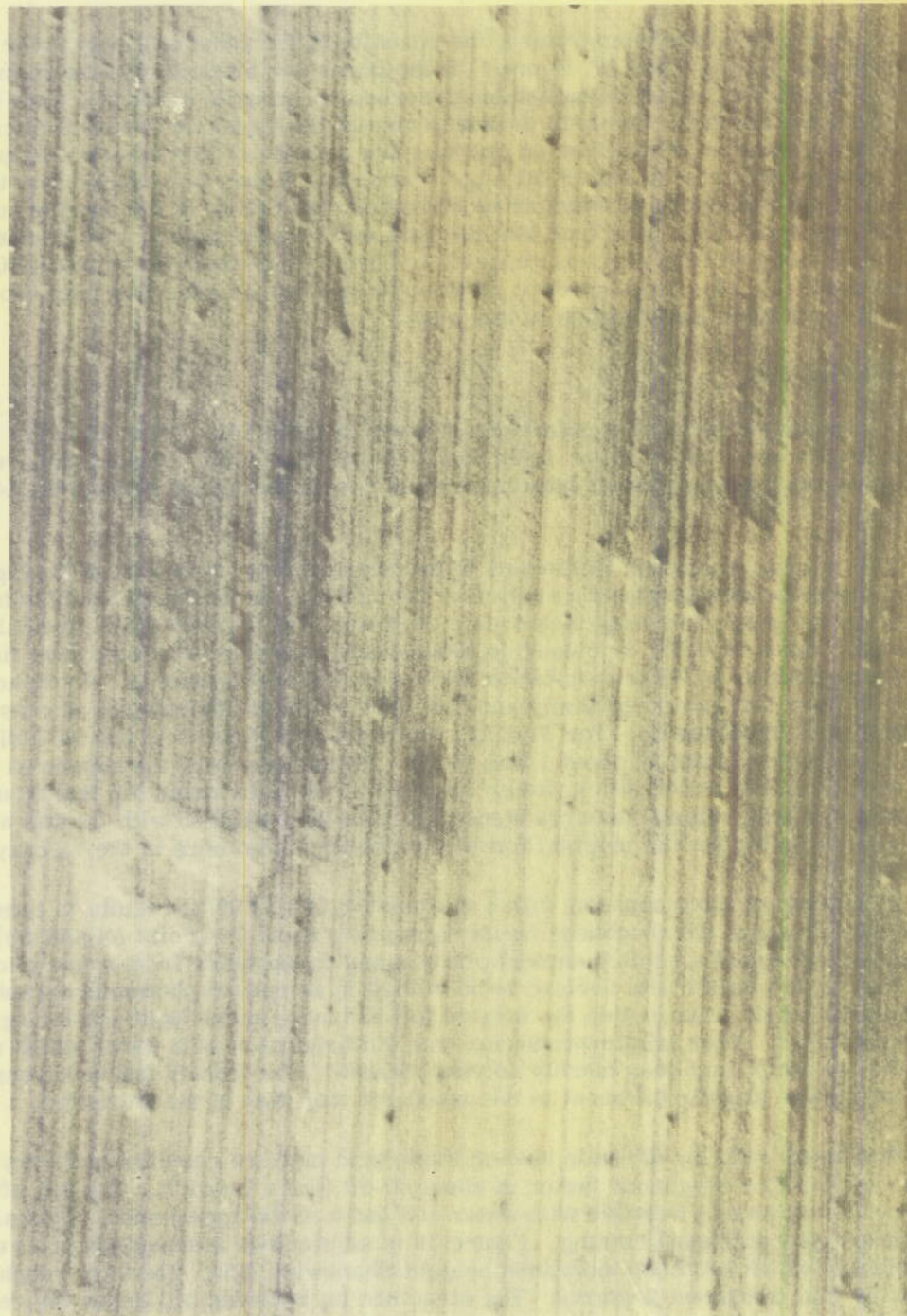
Figure 38 Electron Micrograph of Untreated Aluminum Foil, 8000 X
