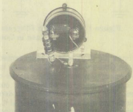
Figure 3 - Crystal Detector Circuit With Shield Removed
