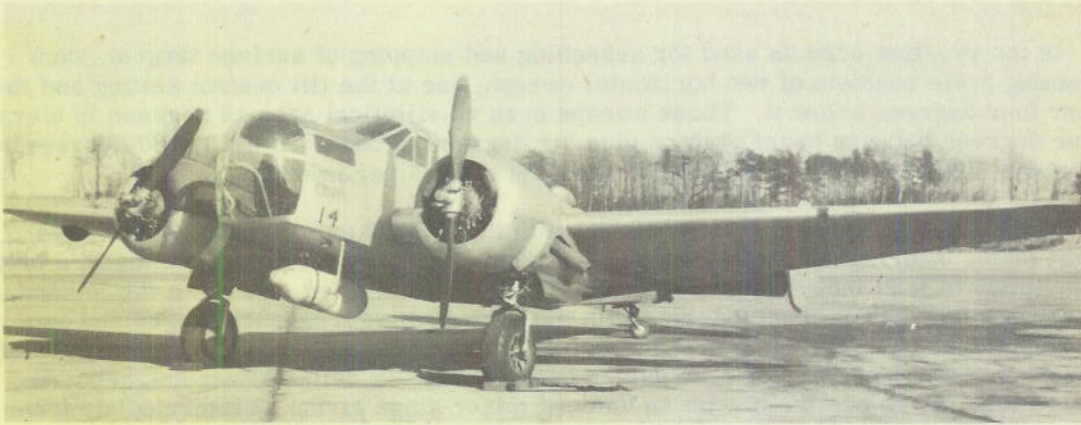
Fig. 26 - Target Plane With AN/APS-4 Radar Mounted Facing Aft
