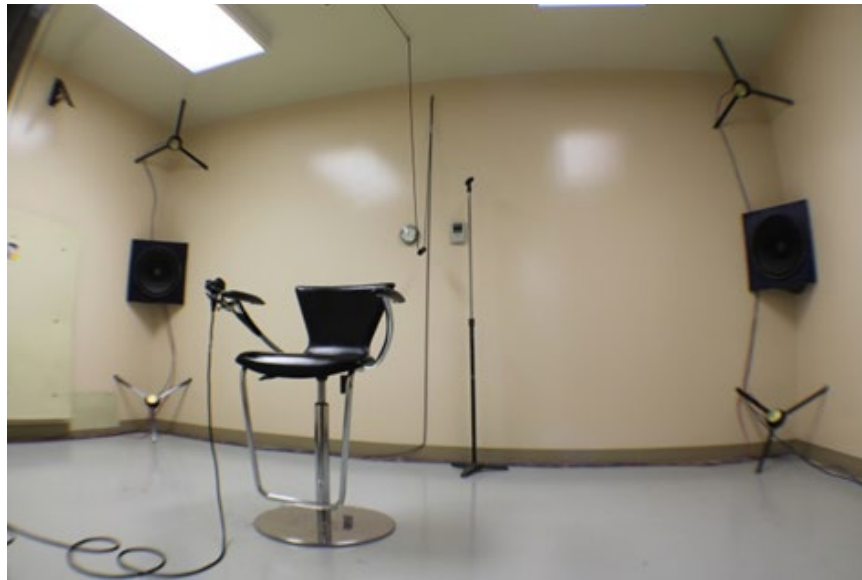
Figure 7. Facility Used for Measurement of Passive Continuous Noise Attenuation.
