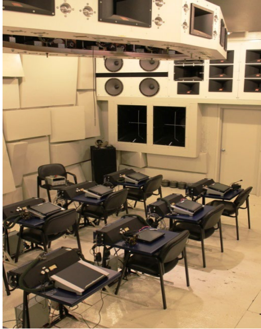
Figure 13. AFRL's VOCRES Facility Used to Measure Speech Intelligibility Performance
