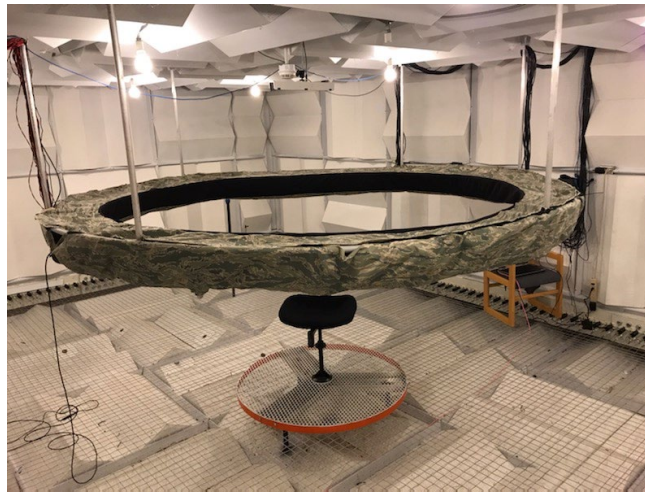
Figure 12. Facility Used for Measurement of Sound Localization.
