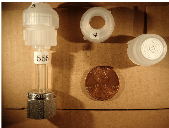
Fig. H3—A close-up photo of the particle collection filter housing. Complete unit at left, with cap removed at right showing filter support. Cap in middle.
