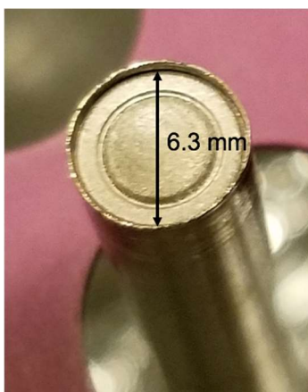
Fig. 20—Metal collection frit (Restek # 25072), mounted on the end of a stainless-steel tube, which is inserted into the lower LEQ chamber to collect particle samples
