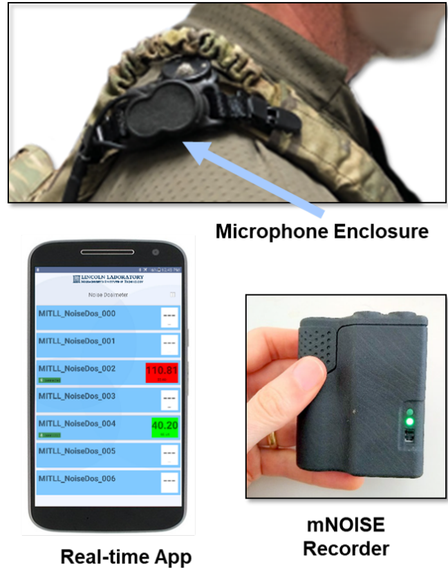
Fig. 1. A photograph of the mNOISE microphone enclosure, recorder, and a depiction of the real-time smart-phone application.
