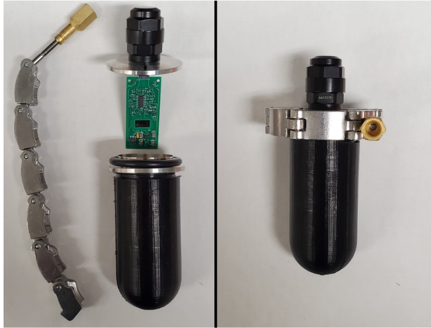
Before inserting sensor into housing (left). Fully assembled sensor in the underwater housing (right). Not shown: addition of the PSF-1cSt silicone oil.
