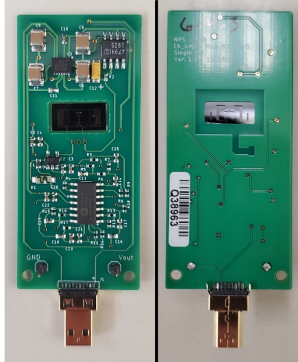
Figure 22. Front (left) and back (right) of a 6-4 sensor attached to a PCB using NOA68 adhesive.
