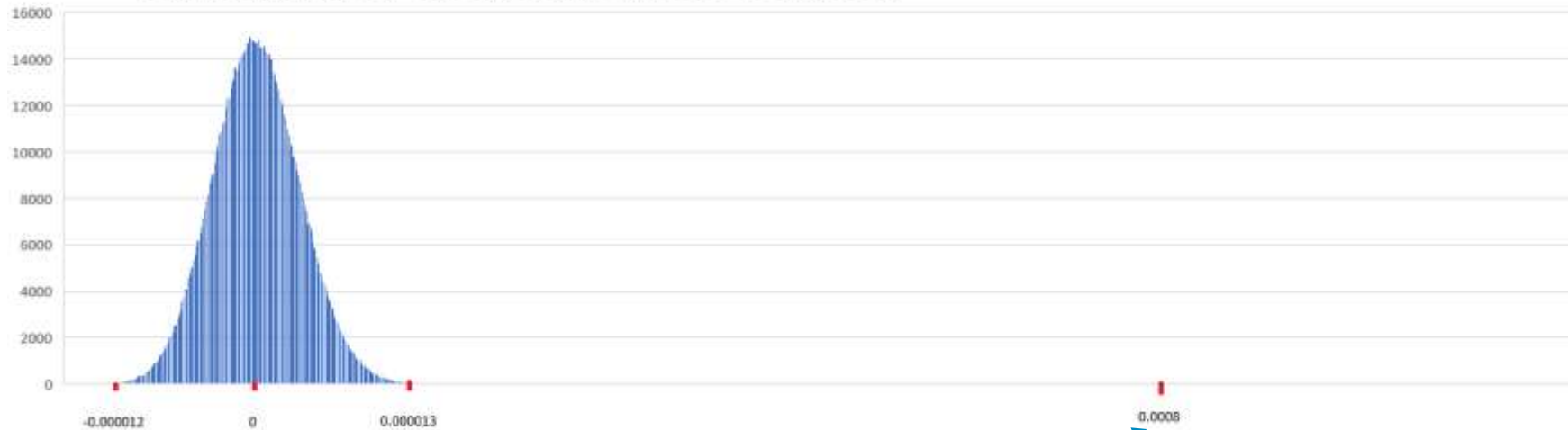
Multiple runs of bubblesort with the same random input: Histogram of deviation of execution time from sample average of execution time (1000000 samples)
