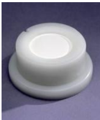
Figure 5-2. Example of a DGT (Diffusive Gradients in Thin Films) device used to measure labile metals in situ .
