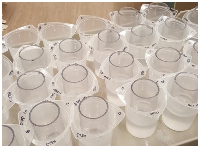
Figure 5-9. Test set-up for sea urchin embryo-larval development pulsed exposure toxicity test.
