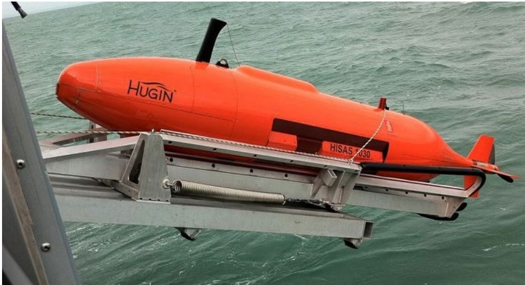
Figure 2 Hugin AUV and recovery system (LARS).
