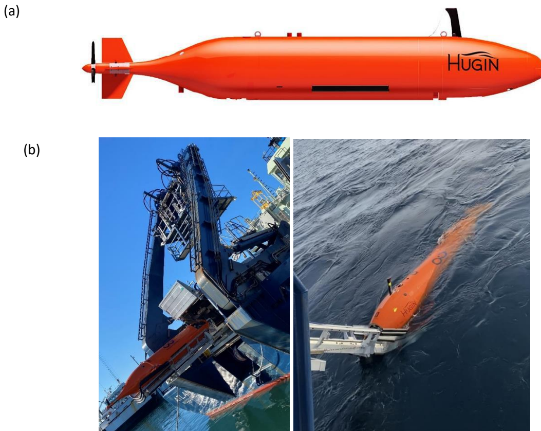
Figure 3. (a) Kongsberg HUGIN AUV, and (b) the deck-mounted launch and recovery system (LARS) The dimensions of the AUV are 6 m long and 0.75 m wide (outer diameters). The AUV was equipped with still image camera, multibeam echosounder (MBES), sidescan sonar (SSS) and subbottom profiler (SBP) for the seafloor survey. The bottom right photo was taken during the AUV was deployed for one of the survey missions on the Atlantis II AUV survey cruise.
