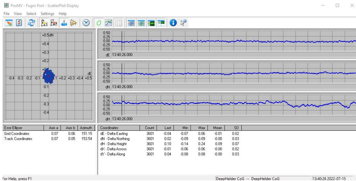
Figure 5 Vessel GNSS static verification.
