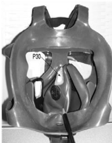
Figure D.49. Inside View of M40 Mask, P30 PAD Location.
