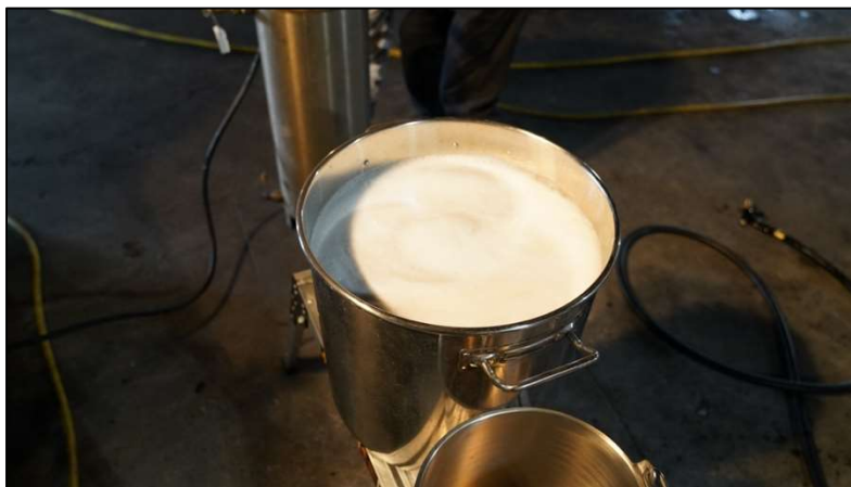
Figure 6: Preparation of the foam solution.
