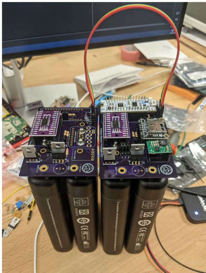
Figure 6-6: Mother/Daughter Battery Monitoring and Control PCBs Each with their 2 Batteries
