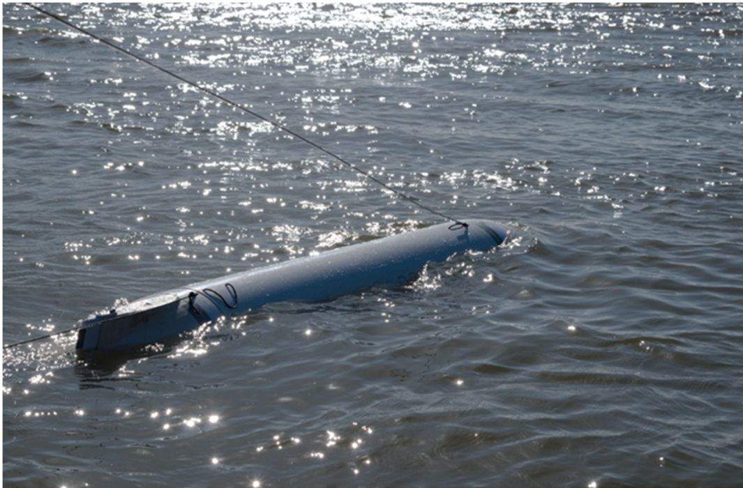
Figure 1-1: The MOANA test AUV which has been configured to test the designed distributed computing and power control system.
