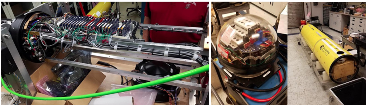
a. Example Mass Slide Actuator for Pitch Control
