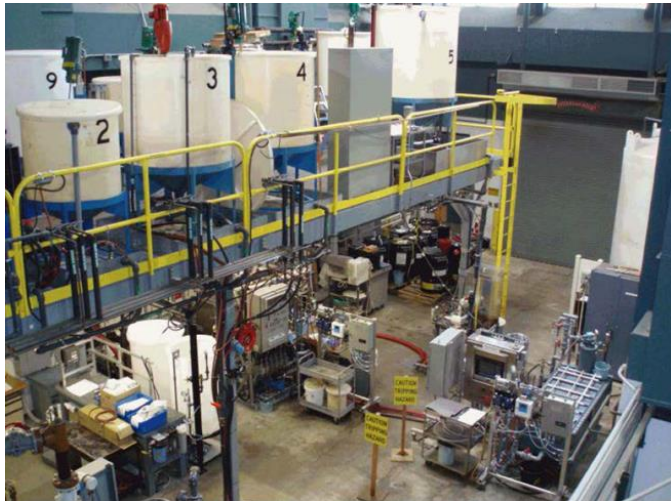
1) Contaminant mixtures and oil prepared and recirculated in upper level-tanks.
