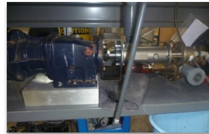
2) Contaminants injected into potable water influent stream using progressive cavity pump or gear pump.
