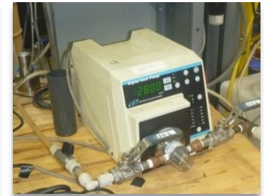
2) Contaminants injected into potable water influent stream using progressive cavity pump or gear pump.
