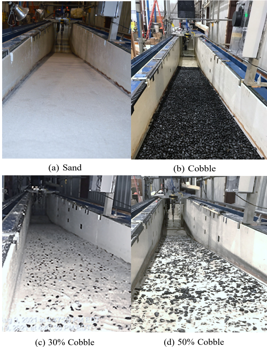
Figure 4: Shown left to right are the four varying beach compositions used throughout the experiment: pure sand, pure cobble, 30% cobble, and 50% cobble on a 1:7 (8 ) sloping beach. Sand was uniformly fine, \phi 0.2 mm diameter and the cobble was 12.7 mm smoothed, black, beach cobble.
