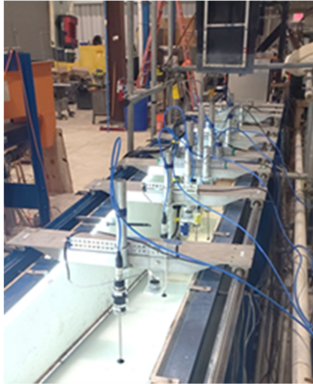
Figure 6: Hydrodynamic station carts positioned at pre-set locations along the length of the flume. Visible carts are equipped with an UDM, ADPV, and EMCM.
