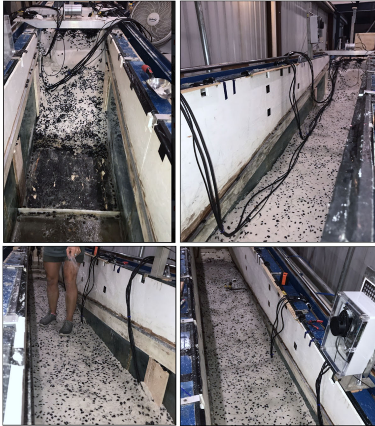
Figure 7: Beach creation process showing the steps for burying the pressure and moisture sensors.
