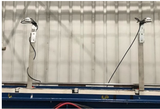
Figure 10: Two of the three RealSense cameras positioned above the flume, oriented downwards.
