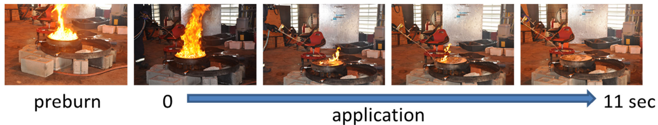
Figure 1 Fire extinguishment experiment with 2062-139/225DK/DGBE in water. The mixture was able to extinguish the 20 square inch F24 pool fire in an average of 11 seconds.
