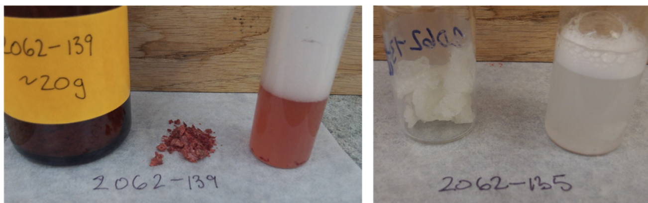
Figure 2 The mono- and bis-gluconamides of diaminoalkylsiloxane 2062-129C and their empirical solubility in water after vigorous shaking.
