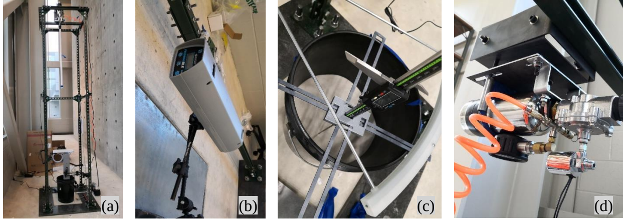
Figure 49. Penetration test apparatus. (a) frame, (b) chronograph, (c) depth gauge, (d) pneumatic launcher.
