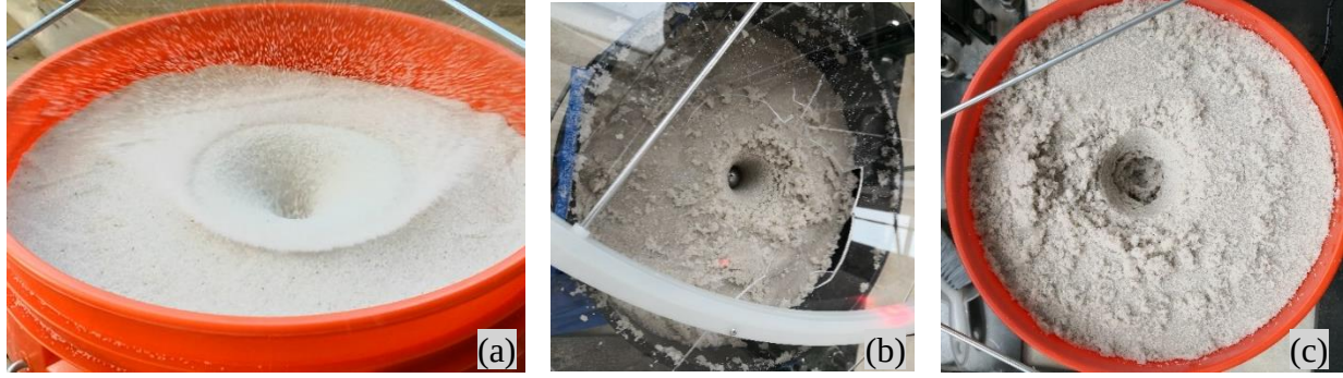
Figure 51. Soil deformations after impact for (a) dry SR=0 , (b) fully saturated SR=1 , and (c) partially saturated SR = 0.5 .
