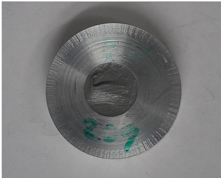
Figure 5 Solder paste sample before reflow.
