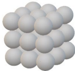
Least efficient stacking (88% of most efficient stacking)
