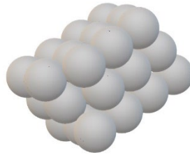
Figure 3 Three point solder ball stacking (3 contact points between all balls with a common void)
