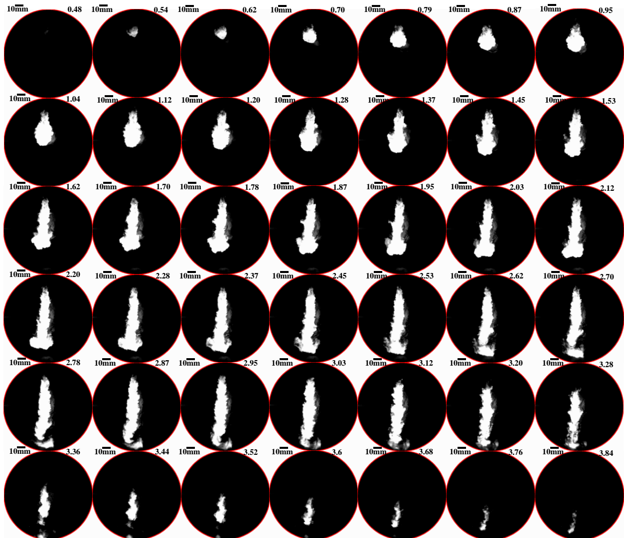
Figure 6: Sequence of images for a typical injection and combustion event. This sequence shows an injection event with the chamber at 60 Bar at 900 K at an injection pressure of 150 MPa. The upper right corner shows time in millisecond after the trigger.
