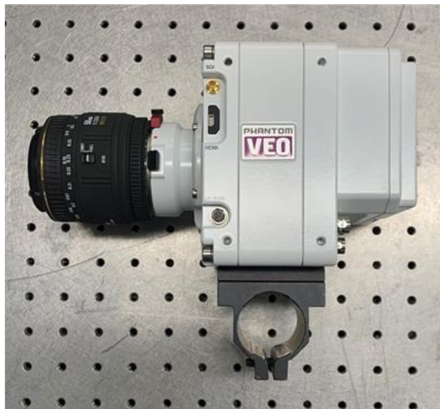
Figure 4: Phantom VEO 710 camera used for the testing.
