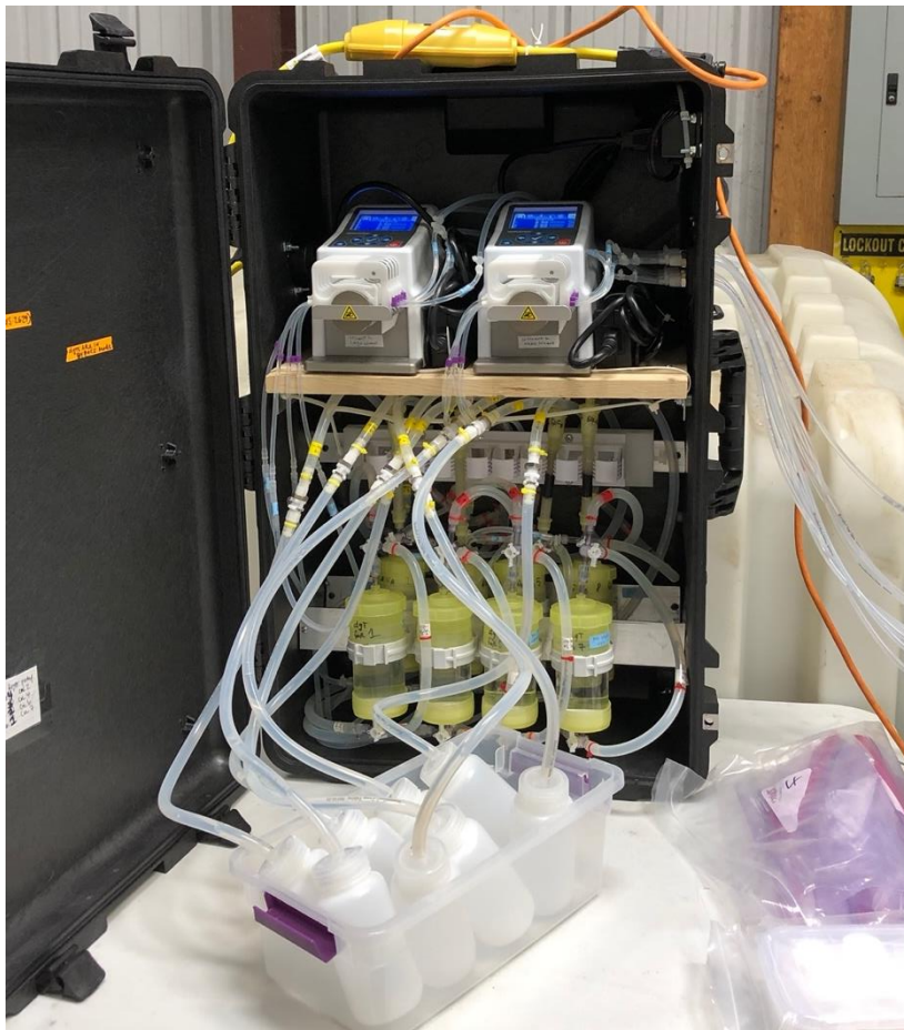
Figure 7: SOTA in operation at field site, during sample collection step.
