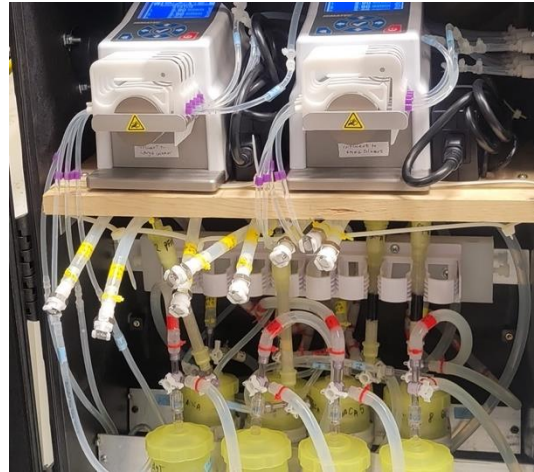
Figure 5: Sample tubes (marked here with yellow zip ties and lab tape) are terminated with female quick-connect adapters and are secured to the bottom of the pump shelf using large zip ties, allowing easy access to collect samples.
