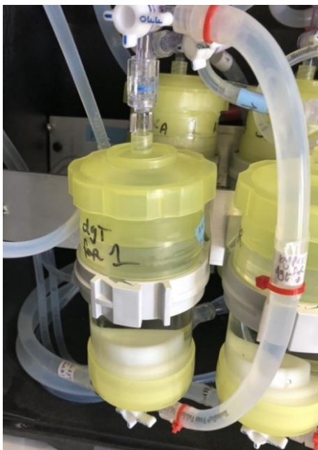
Figure 6: Large column holding a diffusive gradient in thin film (DGT) passive sampler plumbed to receive outlet water from column number 1, with a bypass line (marked with red zip ties) to allow water to continue flowing while DGTs are changed out during the test.
