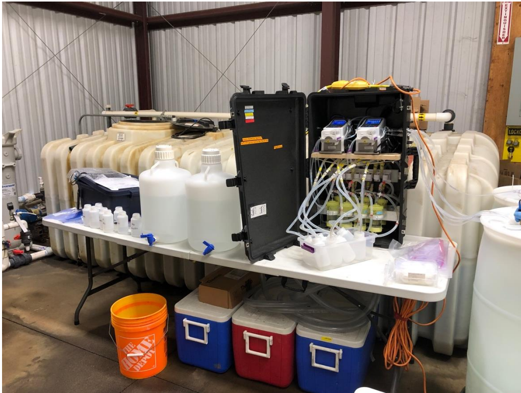
Figure 2: Overview photo of the SOTA (Sorbent Onsite Testing Apparatus) in use at former Marine Corps Air Base Tustin.
