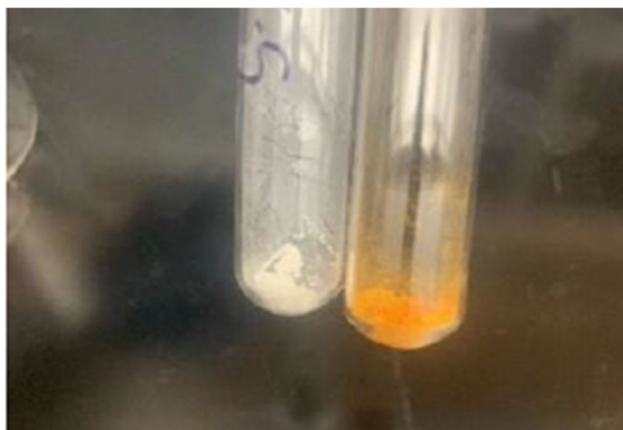
Figure 6. UiO-67.5 Stil (off-white color) and UiO-67.5 Azo (orange) post synthesis and activation.
