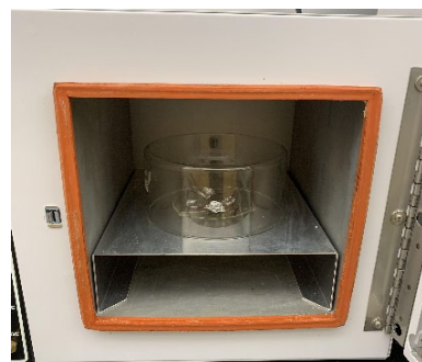
Figure 13. Vapor-Sorption Apparatus in Vacuum Oven.
