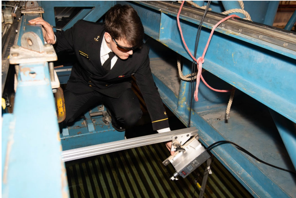
Figure 27: 5W laser being installed onto the 380ft tank Low Speed Carriage.
