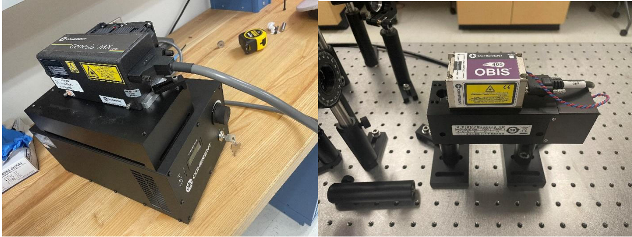
Figure 1.6: On the left is the Coherent Genesis and the right the Coherent OBIS that replaced it. This highlights the size difference and gives a hint at the high power capabilities that we are losing in the swap.
