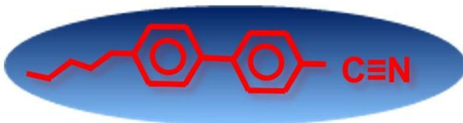
Figure 1: A schematic of an LC molecule, showing a carbon-nitrogen polar bond connected to two benzene rings, followed by a tail of alkyl side chains. The carbon-nitrogen bond gives the LC molecule its polarity, the benzene rings promote attraction between surrounding molecules, and the alkyl side chains assist in elongating the molecule in order to enhance its anisotropic properties.
