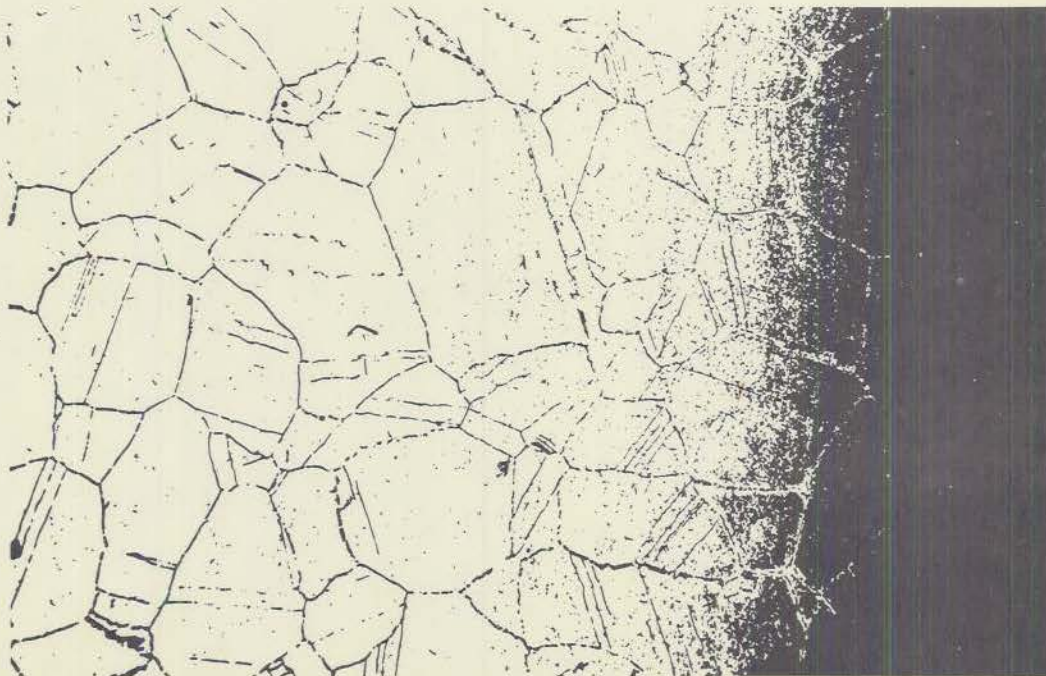
FIGURE 7 (8659) CARBURIZED CASE .004-.006" FOUND ADJACENT TO BLACK STREAK ON I.D. OF TUBE.
