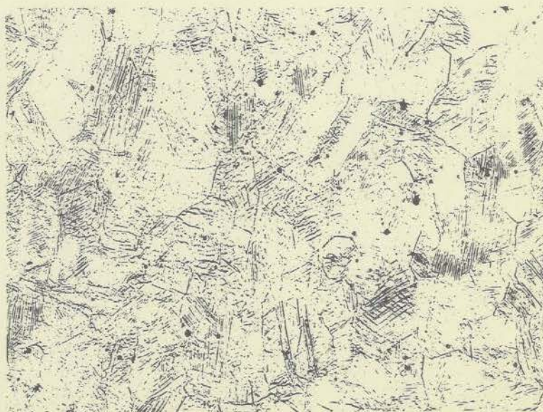
X 100 ETCHANT: OXALIC ACID FIGURE 24 (9073) TYPE 310 BLANK SHOWING STRAINED CONDITION.
