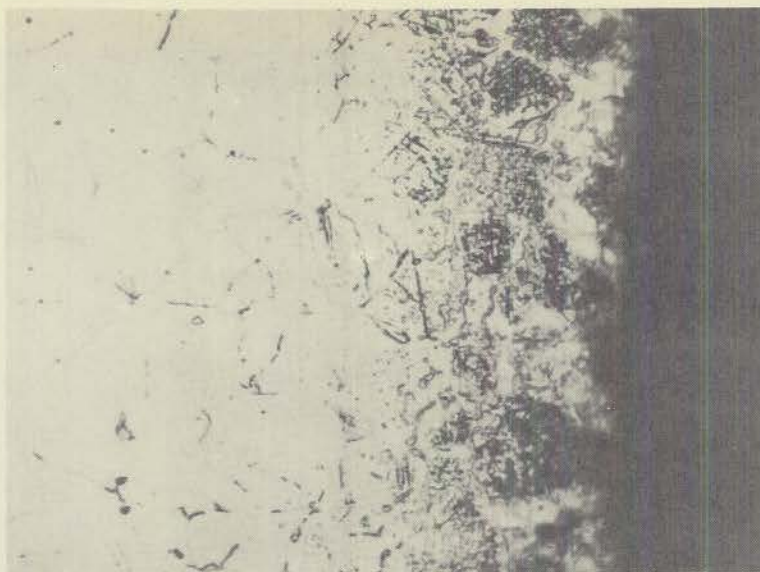
FIGURE 29 (0065) TYPE 304 - STRUCTURE OF K VAPOR SAMPLE SHOWING DIFFUSION ATTACK.
