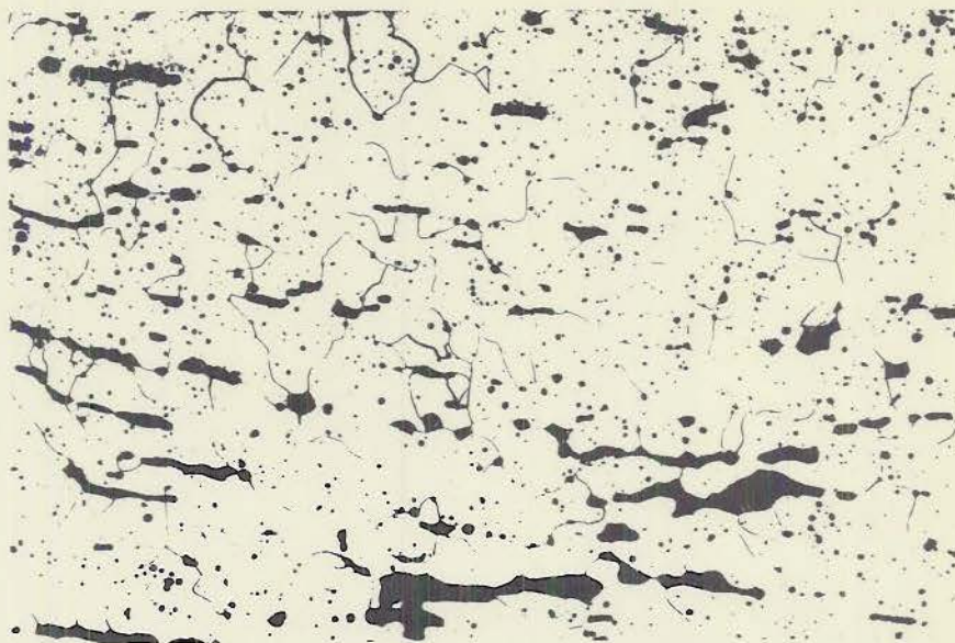
FIGURE 17 (8847) REPRESENTATIVE STRUCTURE OF WROUGHT IRON BLANK.
